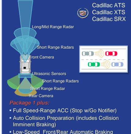
Low-Speed Front/Rear Automatic Braking (Emergency Braking to Avoid Contact)
